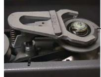
Install the spring fork assembly. Insure the tab on the motor pulley is pointing toward the rear of the mixer.
