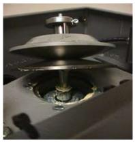
With the new pulley in hand, align the motor key with the key slot in the motor pulley.
