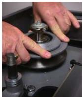
Now, using the upper movable pulley,repeatably "slam" down against the lower pulley. This action will "push" the pulley into place. Continue until the pulley bottoms out on the shoulder of the motor shaft.
