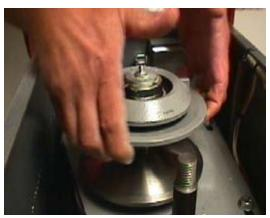
This action will eventually cause the motor pulley to come up and off the keyed motor shaft.
