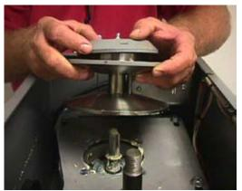
Remove motor pulley.
