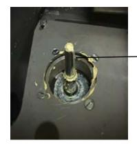
The motor shaft and key.
