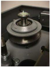
Motor pulley on shaft.
