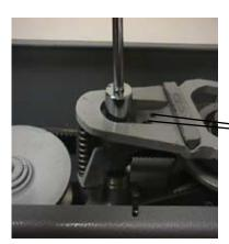
Tighten the 24 MM nut WHILE THE MIXER IS RUNNING. Tighten until the nut bottoms out.
