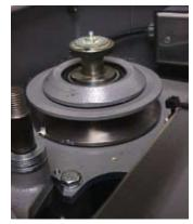
The motor pulley installed.
