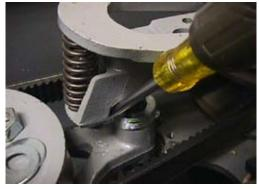
Insert screwdriver as shown, and pry up the spring fork assembly.
